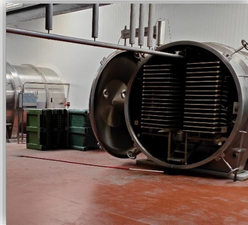
1 of 3 freeze-drying machines at Natures Menu's Snetterton facility
